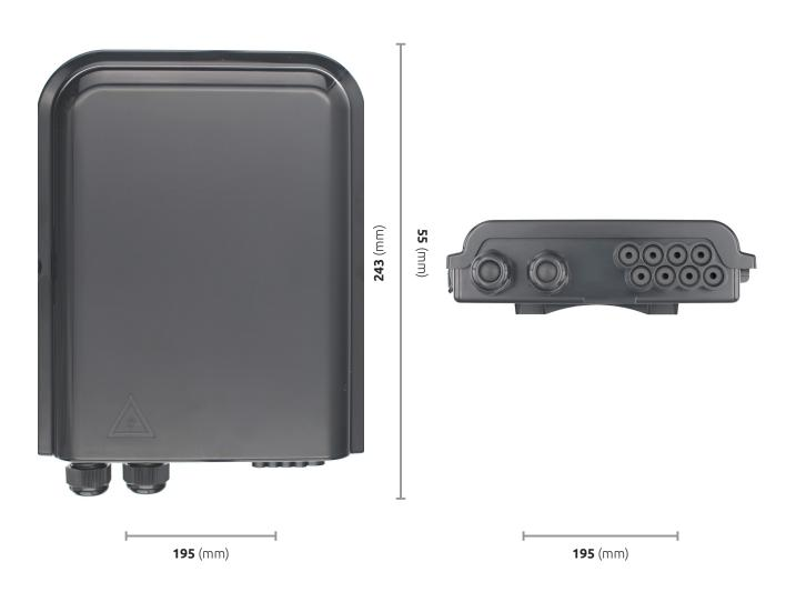
Order Code: BTFAT0311B Type: Fiber NAP Boxes Application: Indoor/ Outdoor use: Splicing / Splitter IN/OUT Ports: 2:8 Inlet/Outlet Caliber: 12 mm / Drop-3.0 mm Max. Splice Capacity: MAX: 8 Dimensions (H\*W\*D): 243 mm \* 195 mm \* 55 mm Operating Temperature: -40 °C to +65 ° C
