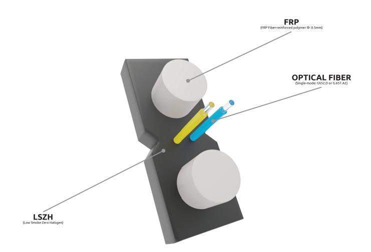
Order Code: BTDFSA Fiber Type: Single-mode: G652.D or G.657.A2 Wavelengths: 1310 nm, 1490 nm, 1550 nm and 1625 nm. Number of Fibers: 1, 2, and 4 strings available Color Coding: EIA/TIA-598 OD of cable(mm): 2.0×3.0±0.02 Test Methodology: IEC 60794-1-E1 / IEC 60794-1-E3 / IEC 60794-1-E4 / IEC 60794-1-E6 / IEC 60794-1-E7 / IEC 60794-1-F1
